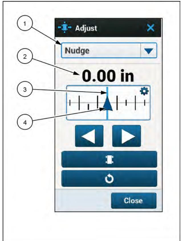
After you apply a nudge, an orange line (1) appears. The orange line denotes the original swath line. The blue line (2) moves to the position you commanded. The blue line represents the desired path for the current operation.
