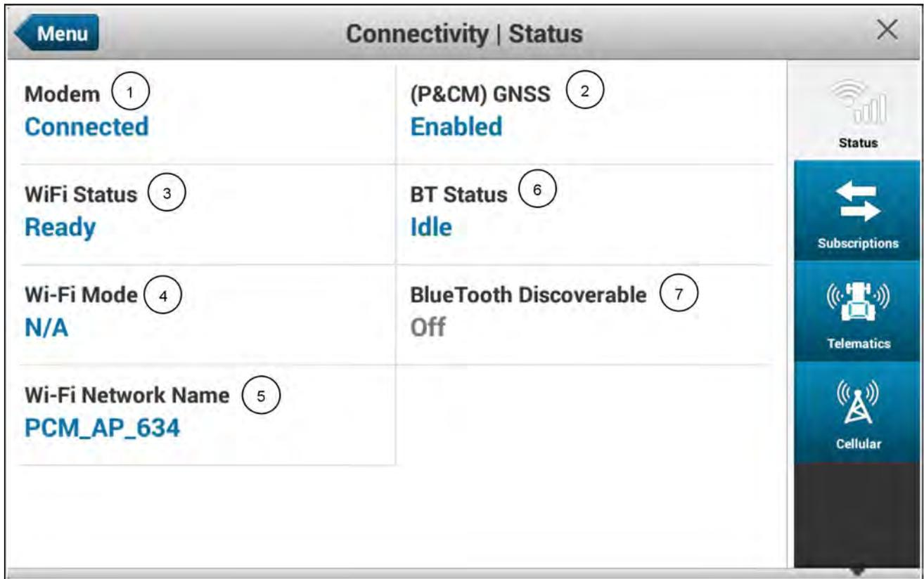
The "Status" screen of the "Connectivity Diagnostics" card displays the following information regarding the Processing and Connectivity Module (PCM):
