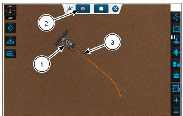
To resume a recording, press the “Record” button on the edit panel which will then change back to a “Pause” button (1). The orange segmented line which was linking the last recorded point to the current position of the recording point on the attachment or vehicle will change back to a dot - dot - dash line (2). The pause icon at the recording point (3) on the vehicle or attachment will change back to a red recording indicator.
