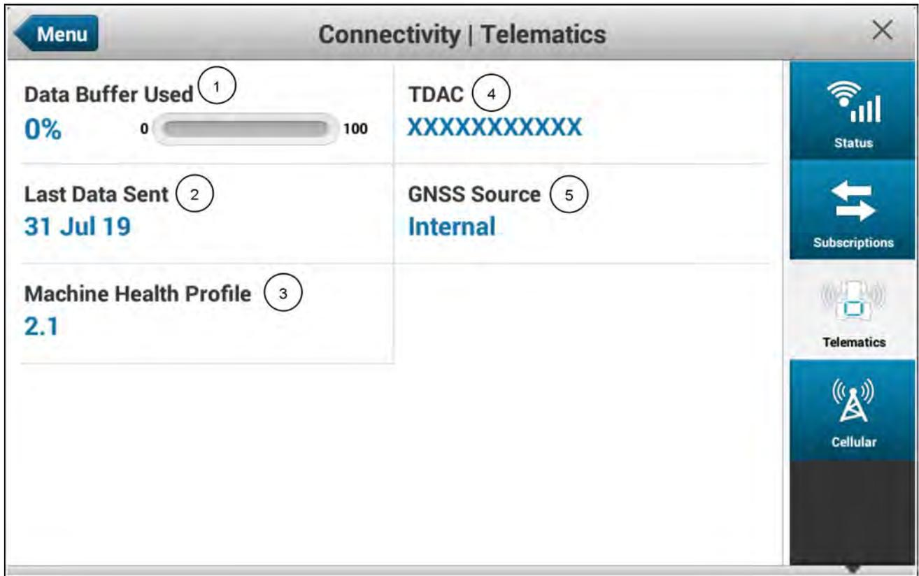
**NOTE:** The basic “Telematics” screen is shown. Depending on your telematics and file transfer subscription level, additional fields described below will be displayed.
