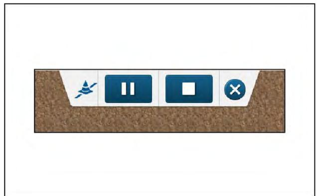
To pause the line landmark recording, press the “Pause” button on the landmark edit panel.
