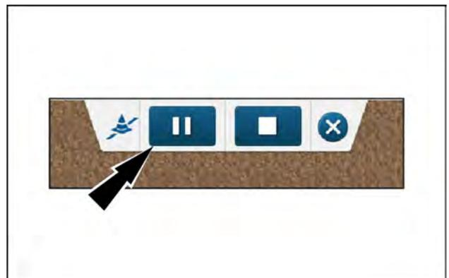
When the pause button is pressed the recording point on the vehicle or attachment **(1)** will update to display a pause status.
