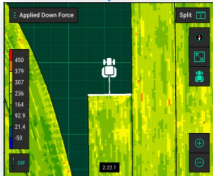
**Down Force** map plots load cell readings on a row by row basis and should be used to set system and monitor performance. A blue dot on the **Down Force** map signifies a loss of **ground contact** which can lead to shallow planted seeds. Blue dots should be avoided and may indicate a higher **Target** is needed, although care should be taken to not over apply downforce. See reverse for more information on **Down Force** settings.
