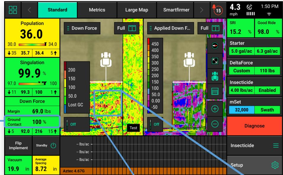
**Target Setting:** If set to **Automatic**, the **Target Setting** will be displayed: **Light**, **Standard**, **Heavy** or **Custom**. Manual setting will display **“Manual”**.
