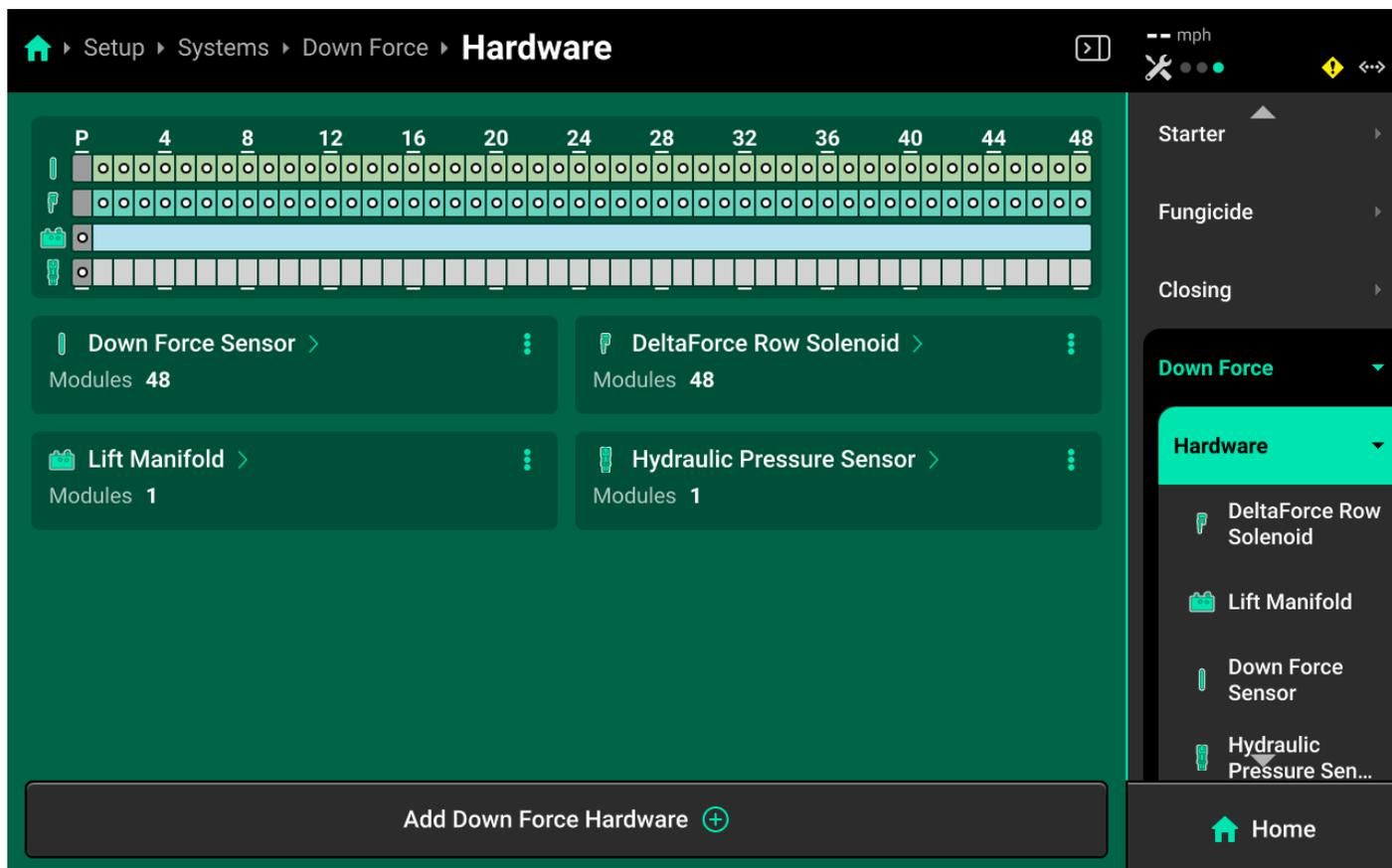
Press the three dots next to any hardware device to delete it or **Edit Locations**, which will run through the setup wizard again.
