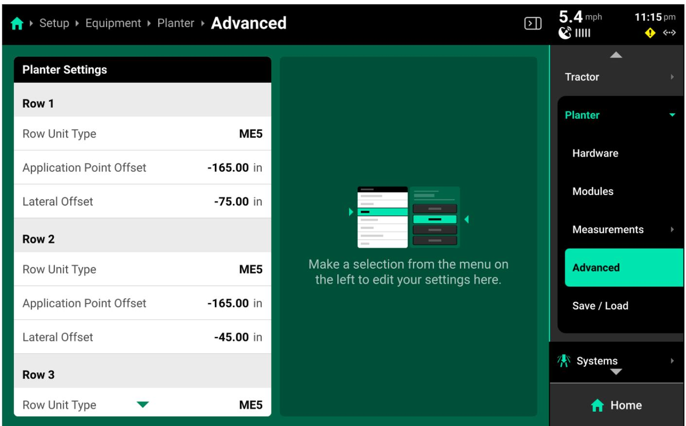
Implements will display the **Advanced** option in the Navigation Menu when **Advanced Frame Type** is selected on the implement profile. The Advanced screen allows the user to set the Row Unit type (planter only) for each row individually. Use this feature on mixed-row unit planters to ensure correct system operation. Ensure to select **Advanced** for **Frame Type / Boom Type** if utilizing the **Advanced** table.
