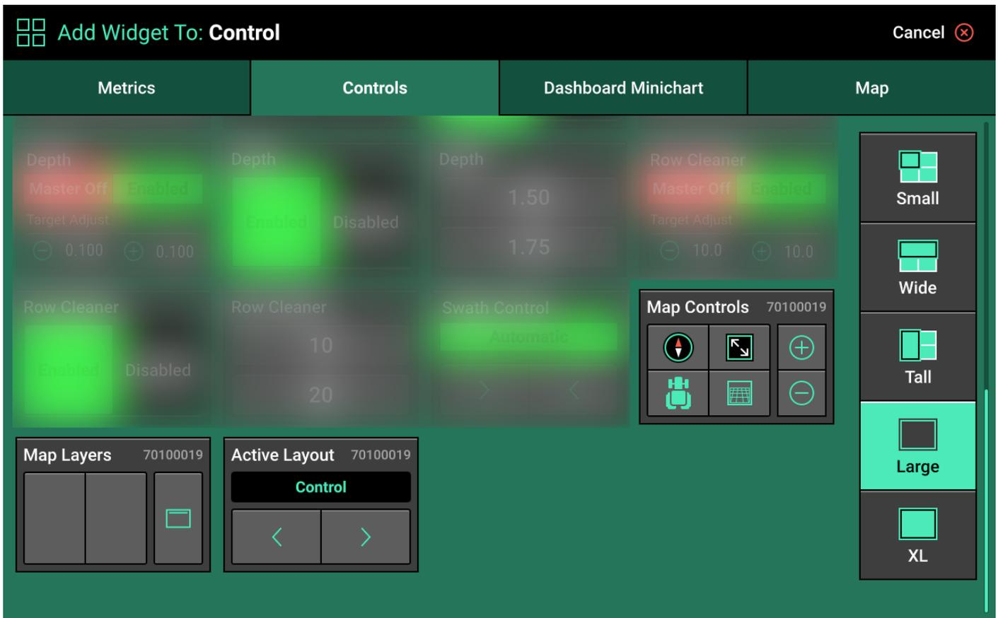
The number in the top right of each widget indicates the serial number of the display that the widget will control.
