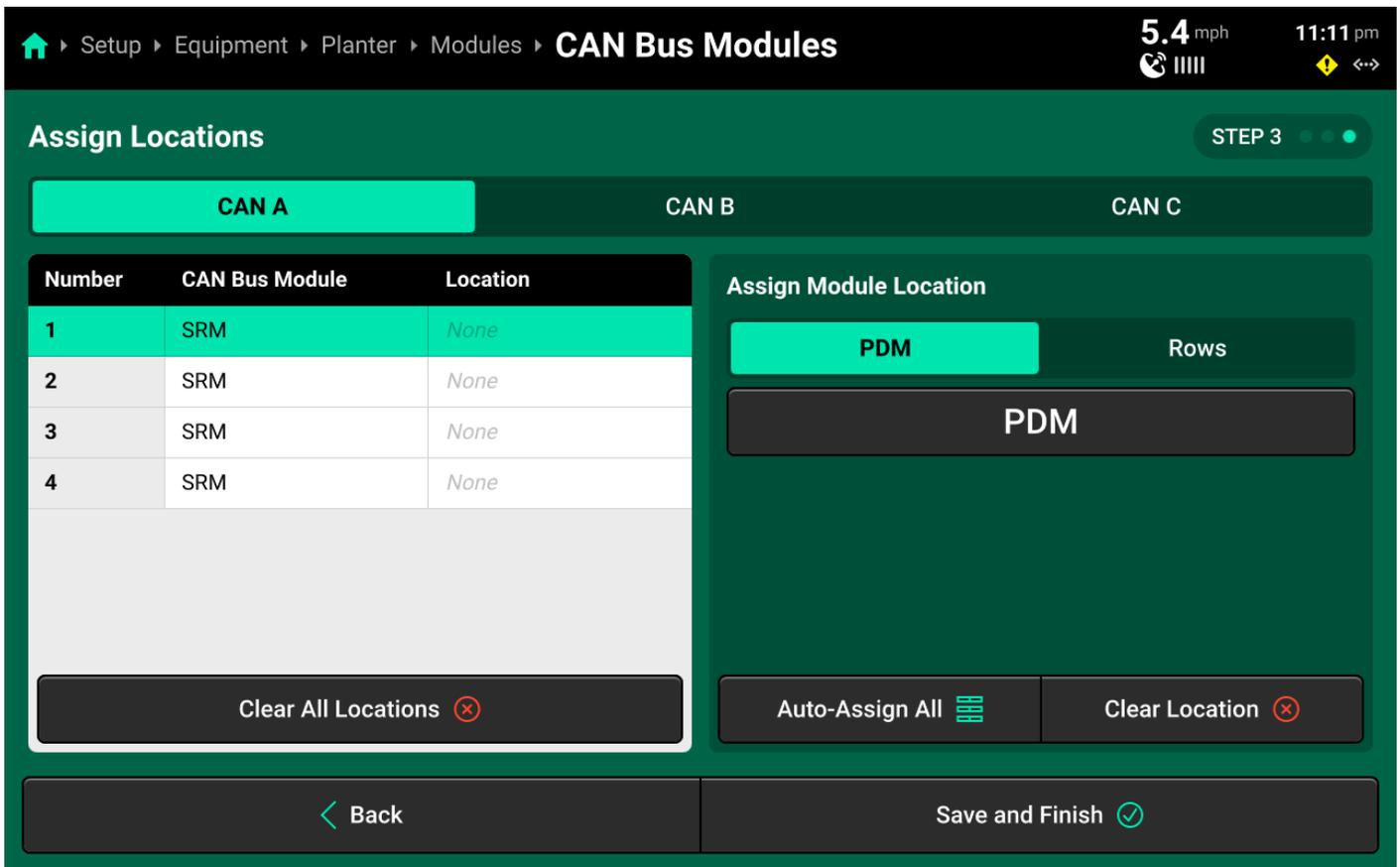
For standard planter configurations, press *Auto-Assign All* in the left window to automatically assign the correct location to each CAN module in sequence, starting with PDM (if set to present) or Row 1 (if PDM is set to not present). Then use the tabs at the top to repeat this process for each CAN bus.
