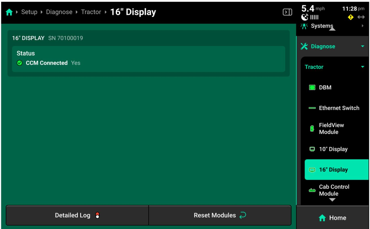
CCM connection status is displayed. Only one display may have a CCM connected. The CCM will be automatically detected.
