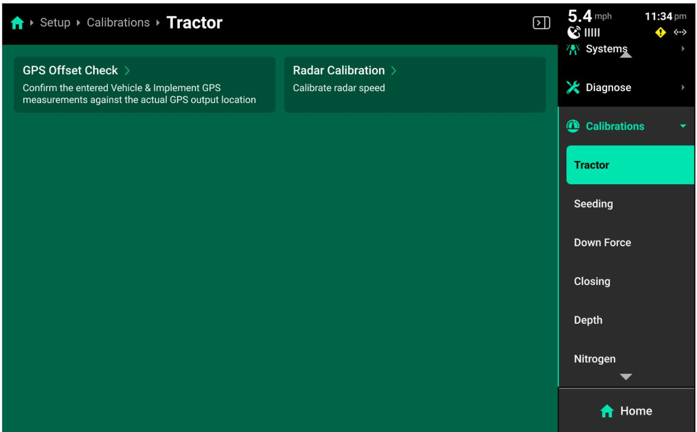
Press (*Cab Name*) in the Navigation Menu to perform a GPS offset check or calibrate radar.
