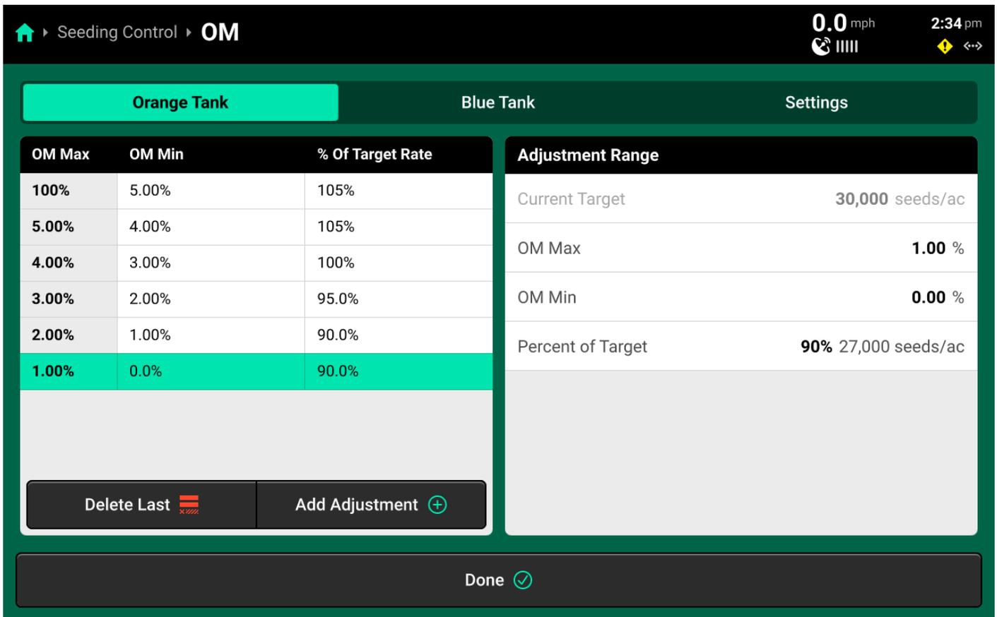
Select a **Range** in the left window, then use the settings in the right window to set values and desired rate for that range. To fine-tune control, press *Add Adjustment +* in the lower left window to add another range. Each range must be configured manually. Use the **Settings** tab at the top to toggle OM / CEC control between Enabled and Disabled.
