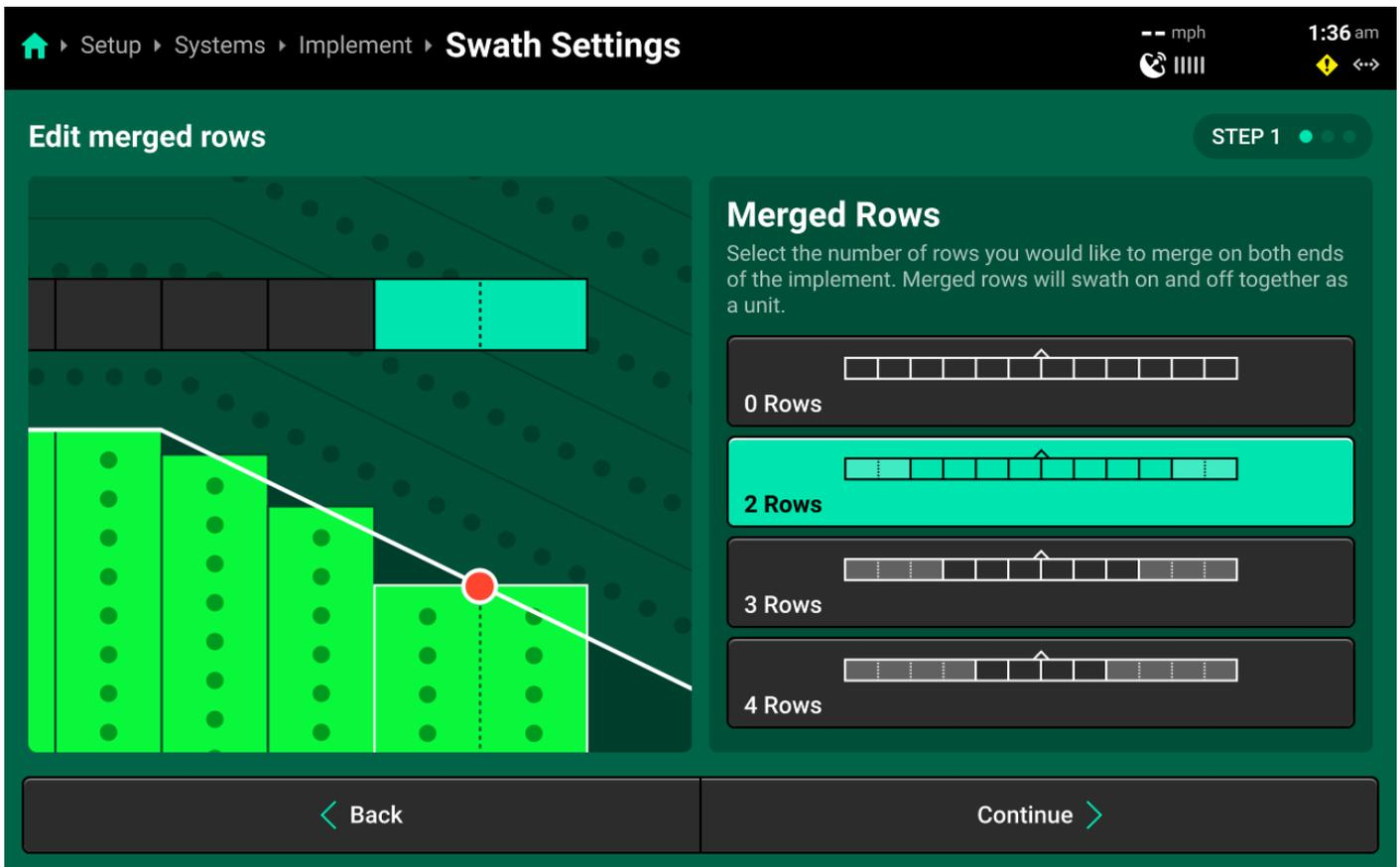
Step 2 (optional) allows the user to enter a positive or negative value to change the point that the 20|20 will use as the center of the merged section. Review choices on Step 3, then press *Save and Finish*.
