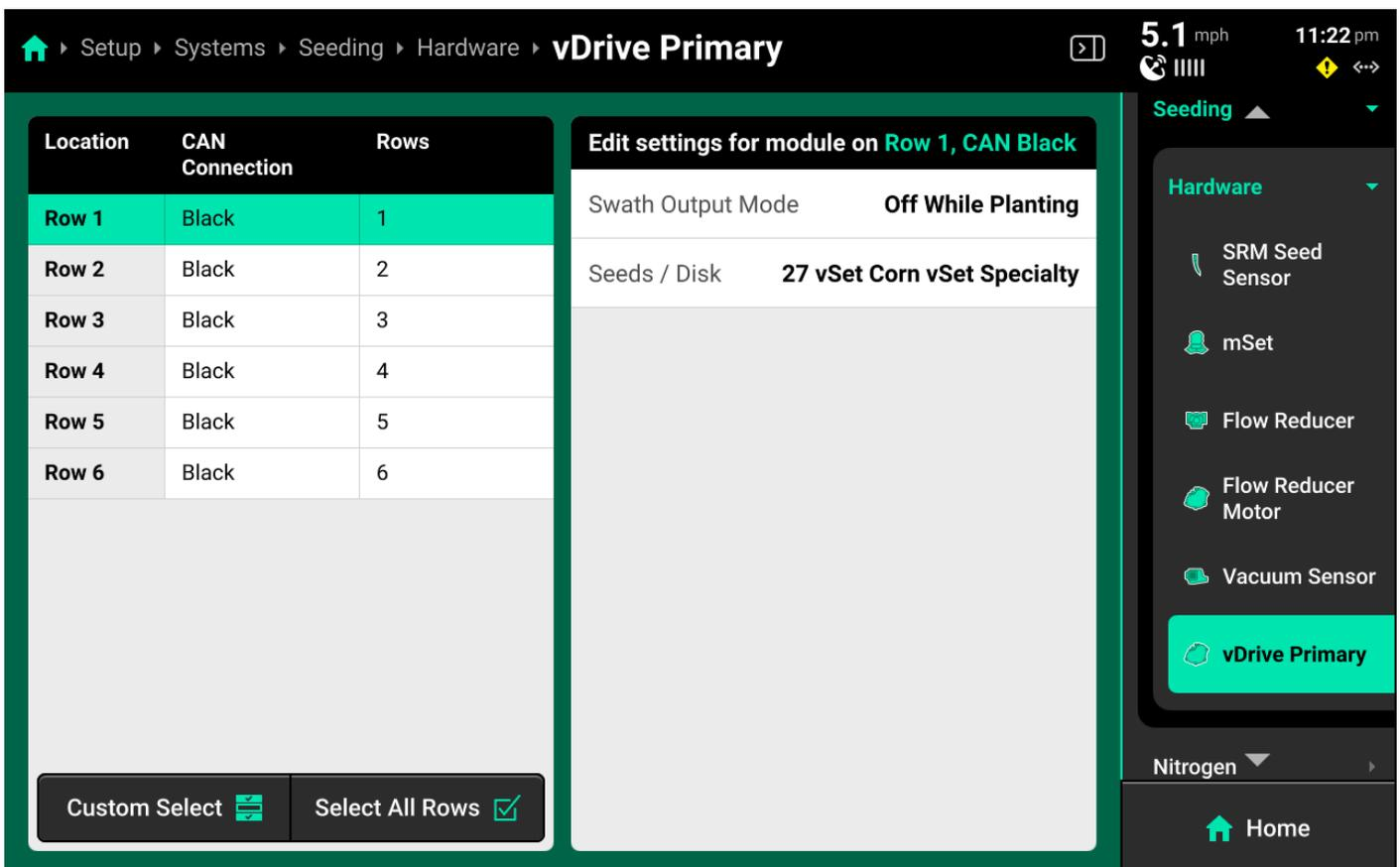
Operation Settings are accessible from the left window of the specific system screen after the hardware device is added. It may be necessary to scroll to view all Operation Settings.
