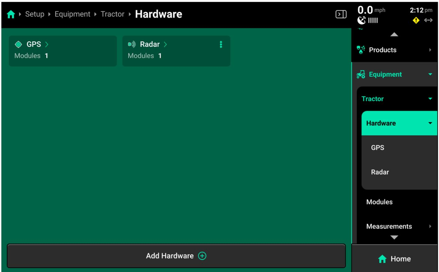
Use the **Hardware** screen to configure GPS receiver or Radar location by pressing *Add Hardware +* at the bottom and following the setup wizard. Press the three dots on any hardware device in the center of the Hardware screen to run the setup wizard again with **Edit Locations** or to delete it.
