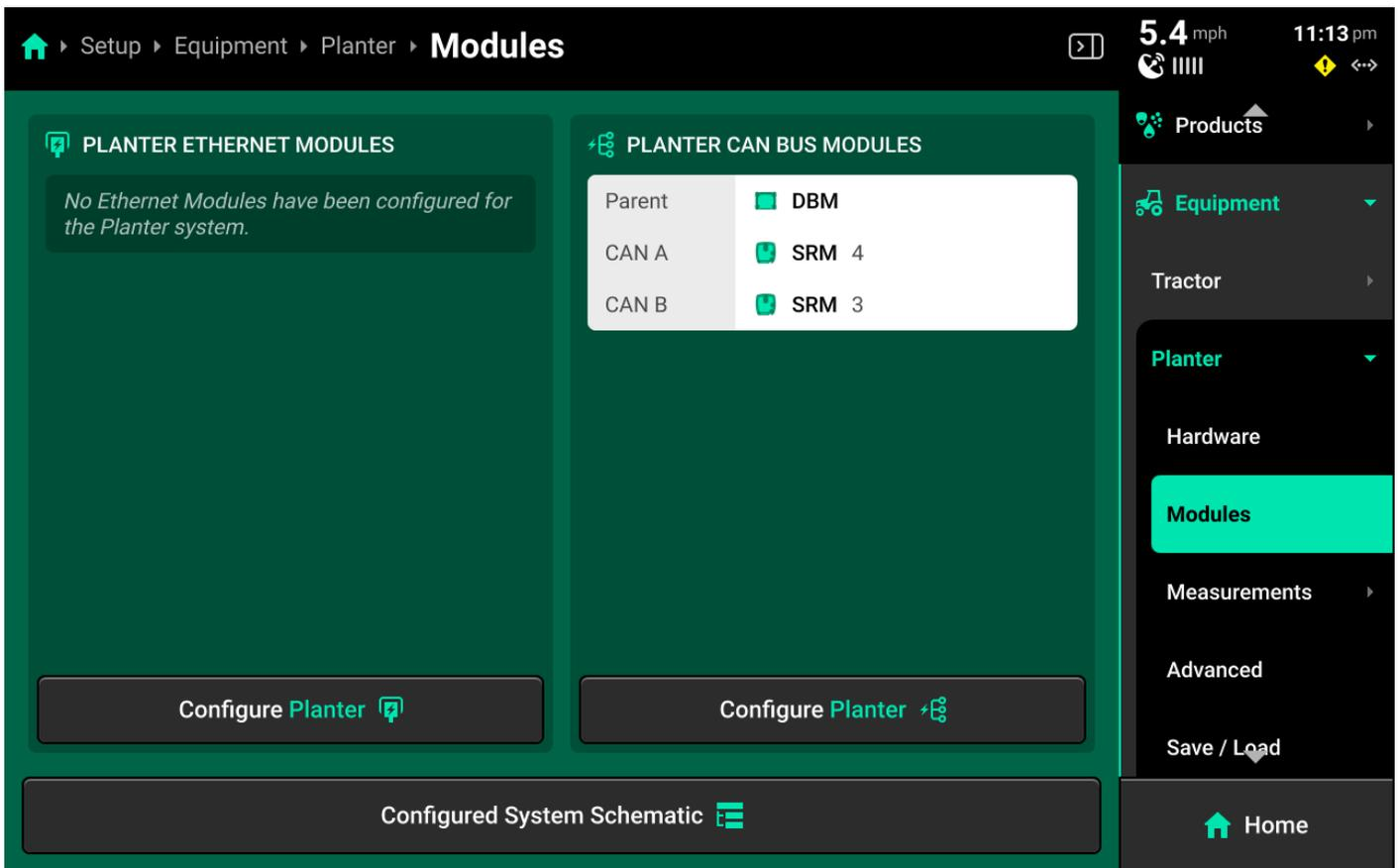
Press *Configured System Schematic* at the bottom to view a schematic of the configured CAN bus(es)
