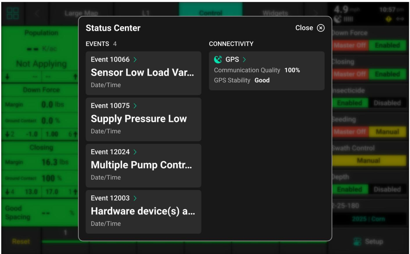
Press any of the events to open a detailed description of that event. Press GPS to navigate to the GPS section of the Diagnose screen. See **GPS** in the **Diagnose** section of this guide for more details.
