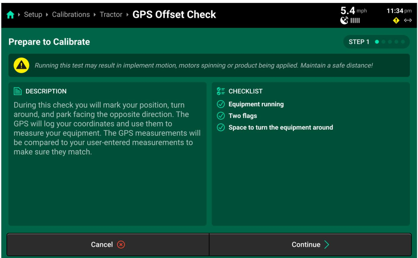
Run through the calibration wizard to perform the offset check following the on-screen instructions. Ensure that the application points / seed exits are even with the placed markers on step 1 and step 4.
