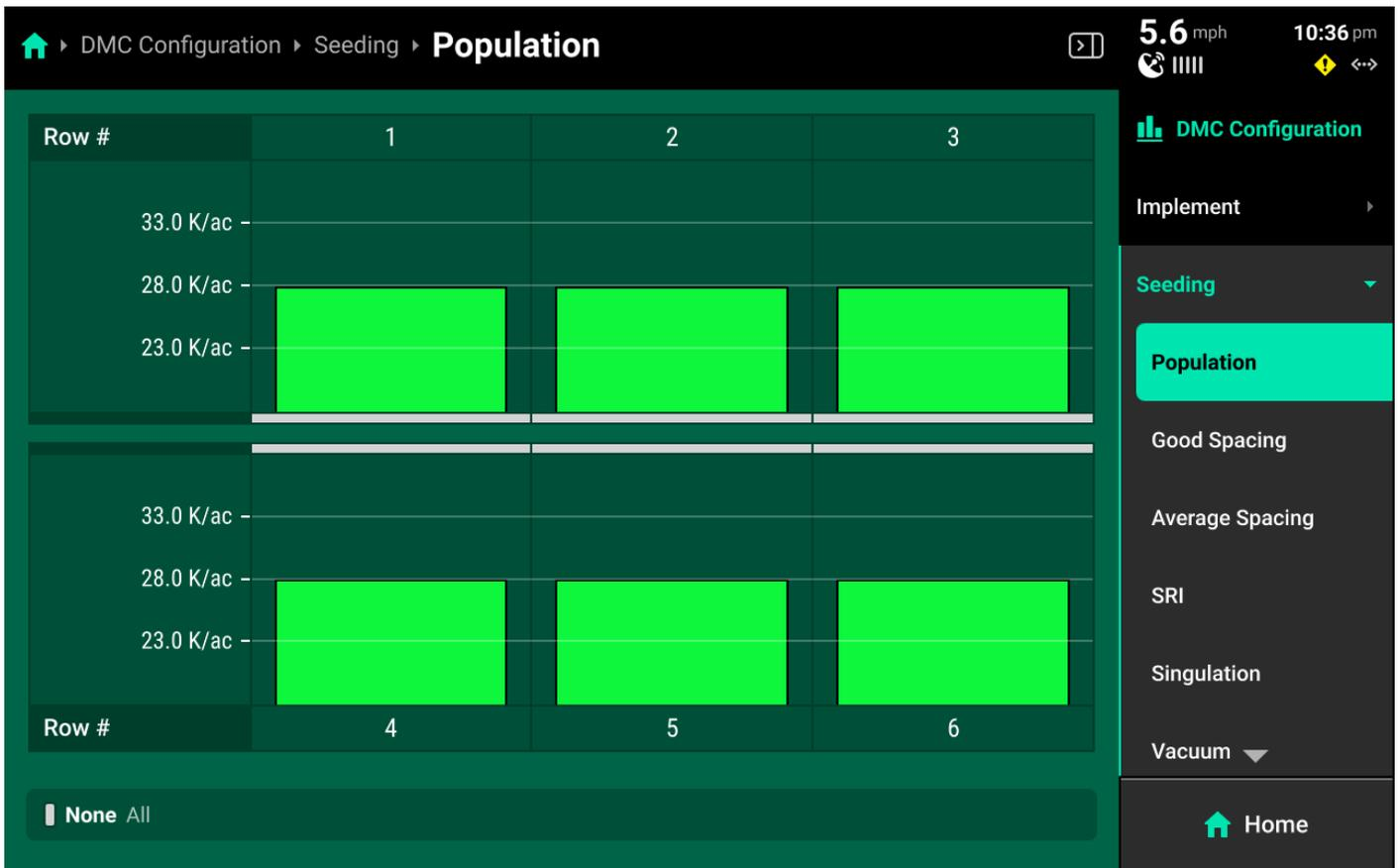
The Metric screen displays a more detailed row-by-row chart. Press any option on the right to view the row details screen for the selected system metrics. Scroll on the menu to view all available options. For applicable metrics, use buttons at the bottom of the screen to scroll between rows or to select a specific row.
