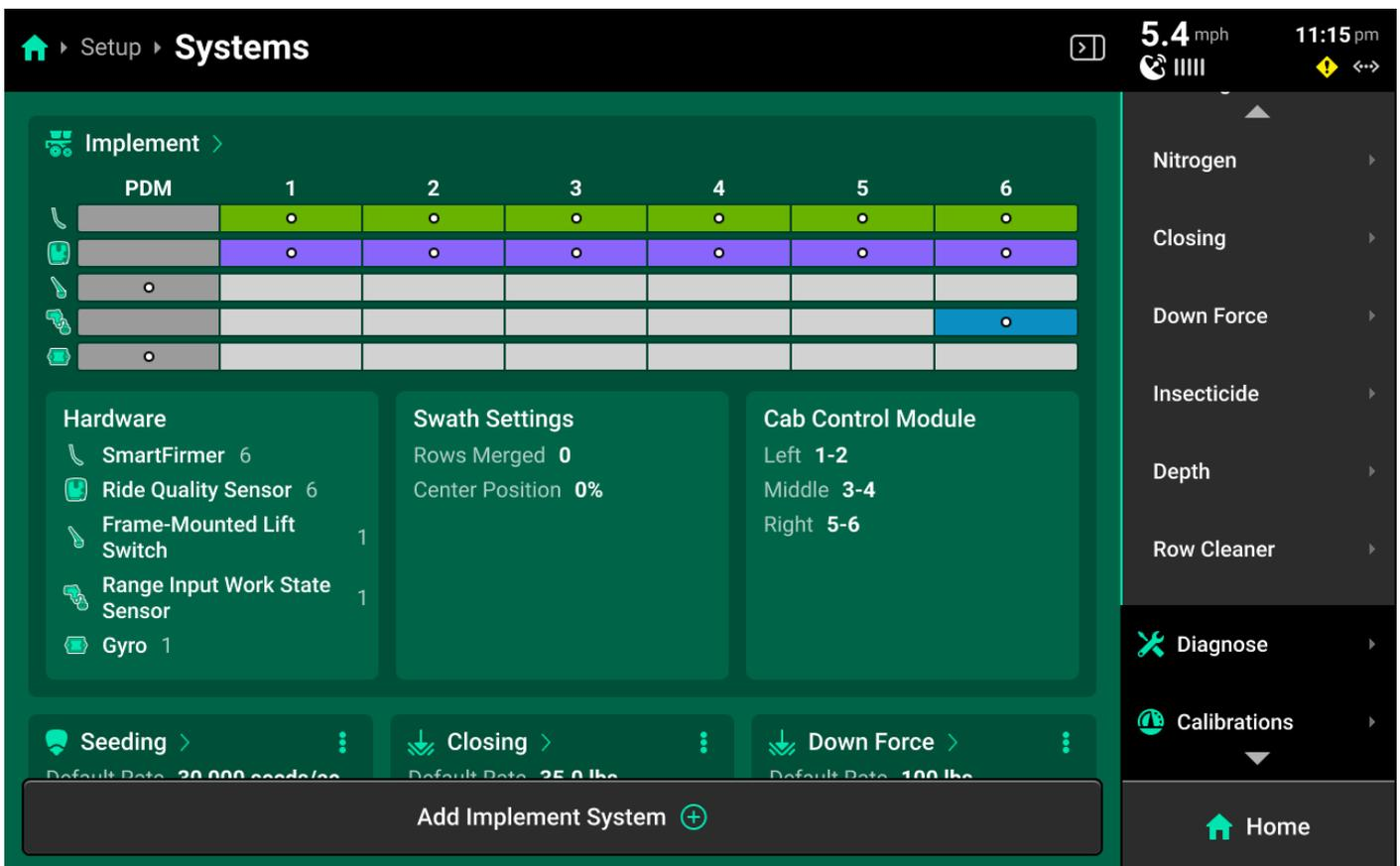
There will be a default system which is either named after the type of Implement profile selected in **Equipment**, or simply titled **Implement**. This system is where all implement-wide hardware, such as lift switches and SmartFirmers, will be configured. All other systems must be added by pressing *Add Implement System* at the bottom of the **Systems Landing Screen**.
