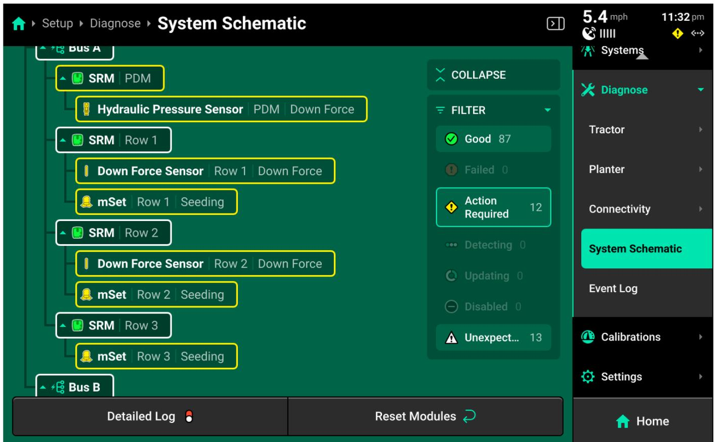
Press the filters on the right side to filter all modules by health. Any filter which is active will have a blue-green outline. Press any active filter to deactivate it.
