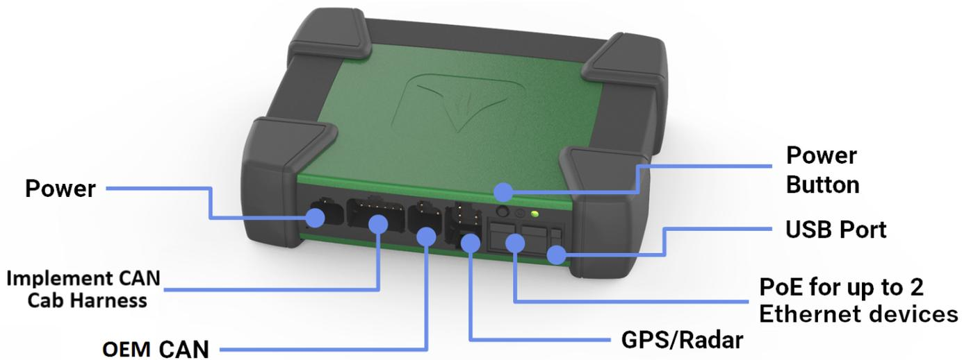
The DBM Power over Ethernet [PoE] ports require a Shielded Twisted Pair [STP] CAT6 Ethernet cable to connect an Ethernet device to the DBM. The different Ethernet devices that may be connected to the DBM are the 10" display, the 16" display, the FieldView Module, and the Ethernet Switch.
