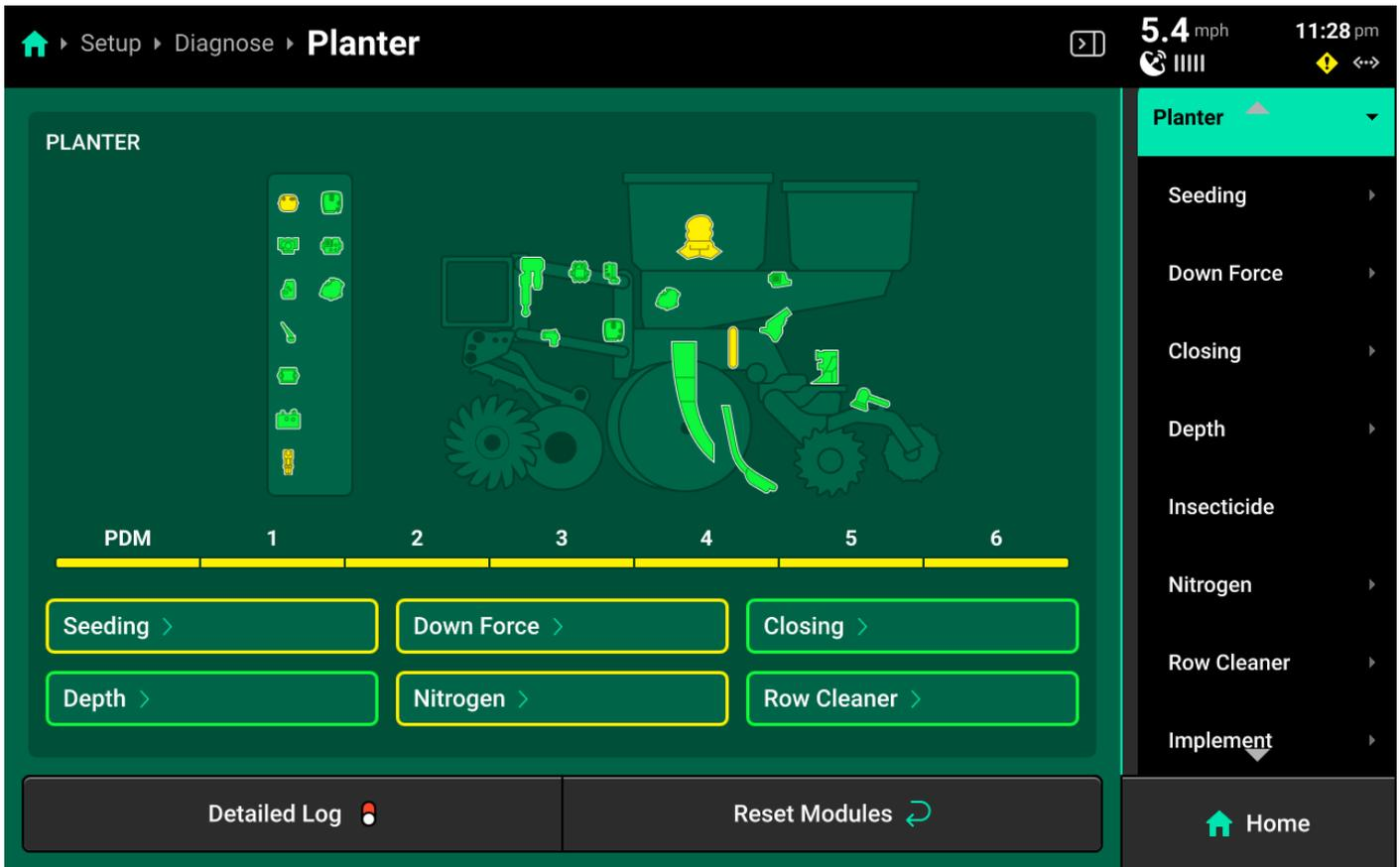
The **Implement** section of the diagnose menu will share the same name as the Implement profile that is selected in **Equipment**. A graphic of the implement and all devices / modules that are installed on it will be displayed.
