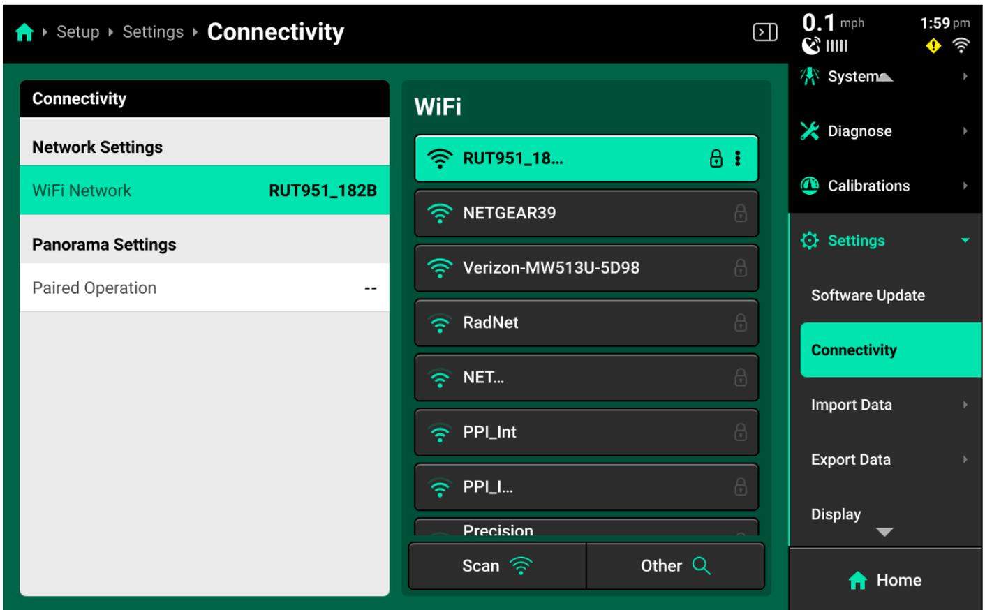
Use the **Connectivity** screen to connect to Wi-Fi or pair the 20|20 with a Panorama operation.
