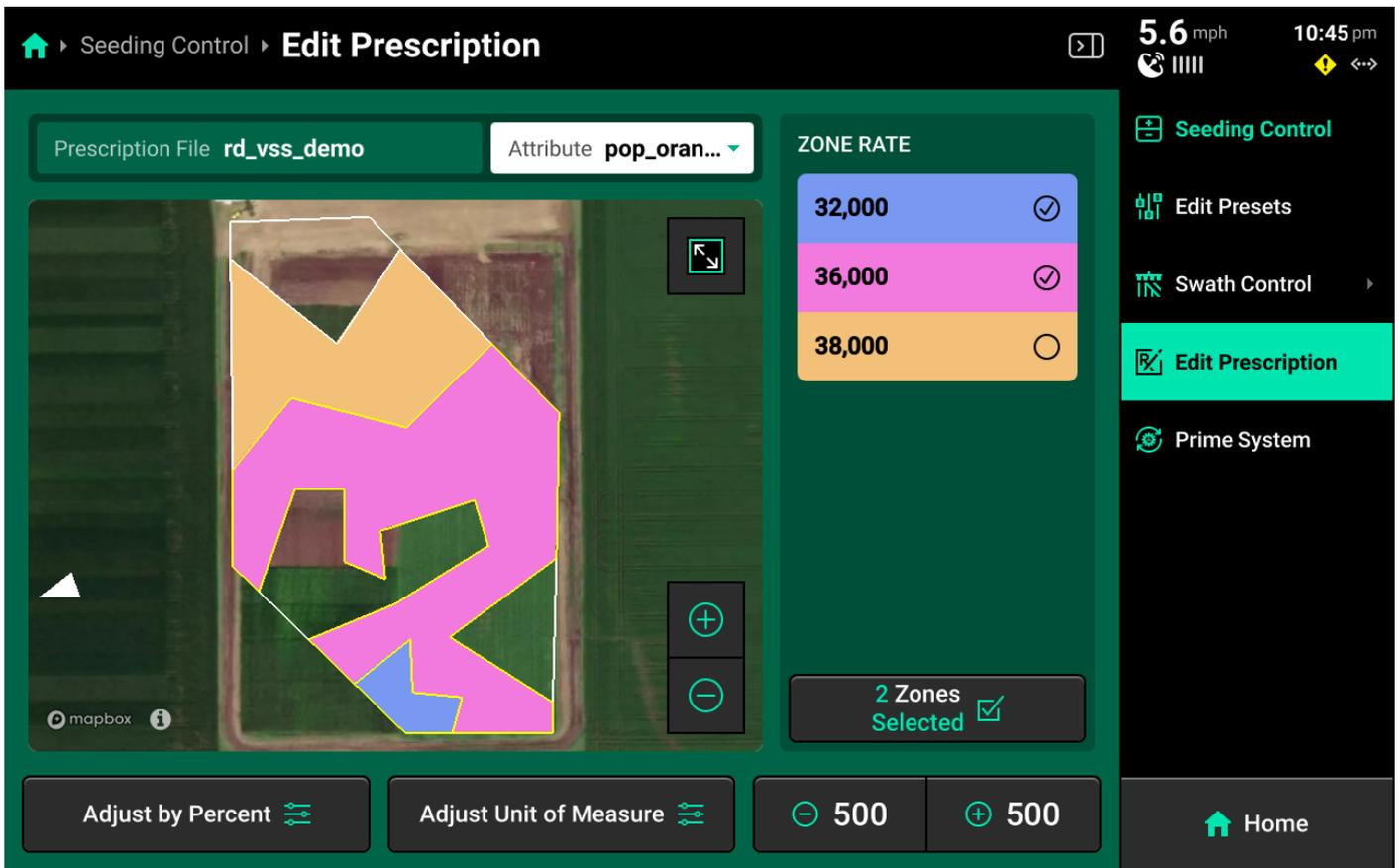
Select the desired attribute to edit using the dropdown box above the map, then select the desired zones rates and use the buttons at the bottom to adjust those rates by a percent or by a preset value. Press *Adjust Unit of Measure* to switch between Imperial and Metric measurements for the selected zones.
