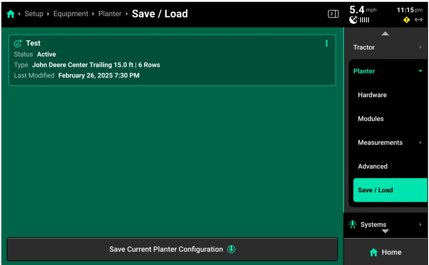
Use the **Save / Load** screen to save, update, and quickly switch between different Implement profiles. A table of all saved profiles of the current type are displayed in the center. Press *Save Current (Equipment Name) Configuration* at the bottom to save the current Product / Equipment / System / Home Screen configurations with the desired name.
