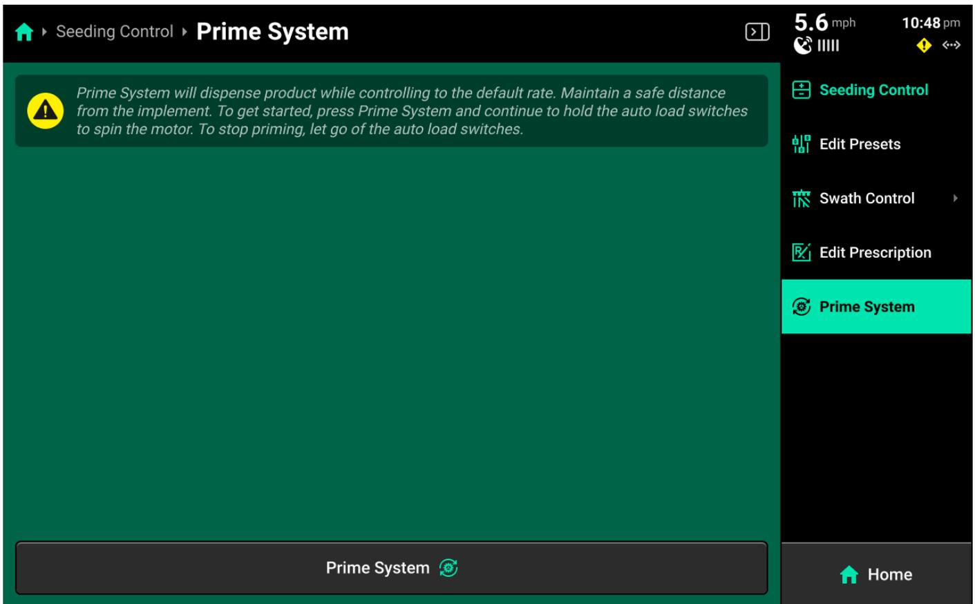
Press *Prime System* on the right to access the **Prime System** function. Press *Prime System* at the bottom of this screen to open a popup which instructs the user to hold both switches up to dispense product at the system's default rate. The system will dispense as long as the switches are held up.
