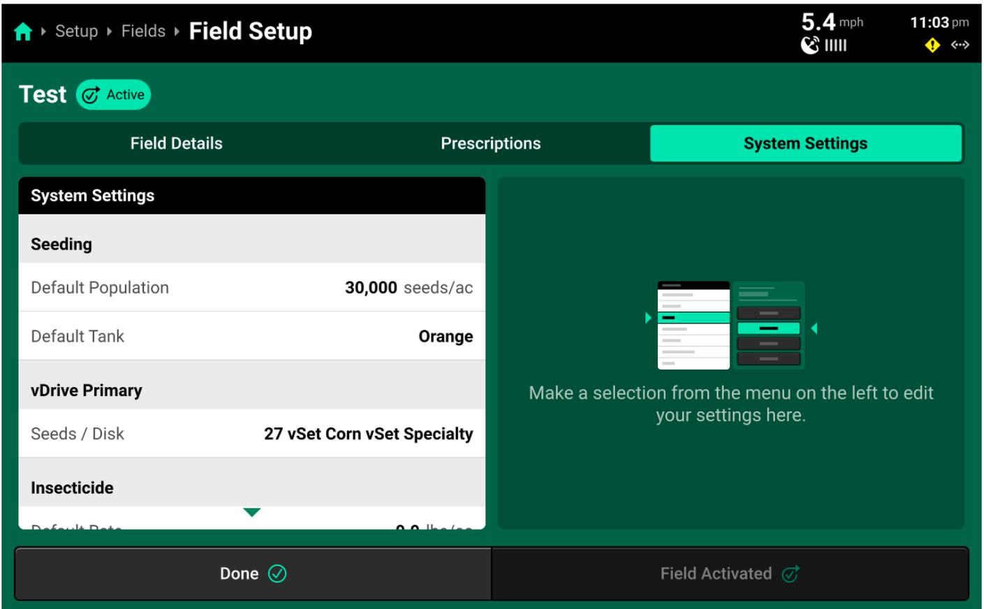
Use this tab to change **Operation Settings** for different system hardware devices, such as seeds/disk. Changes made here will apply to all hardware devices across all rows.
