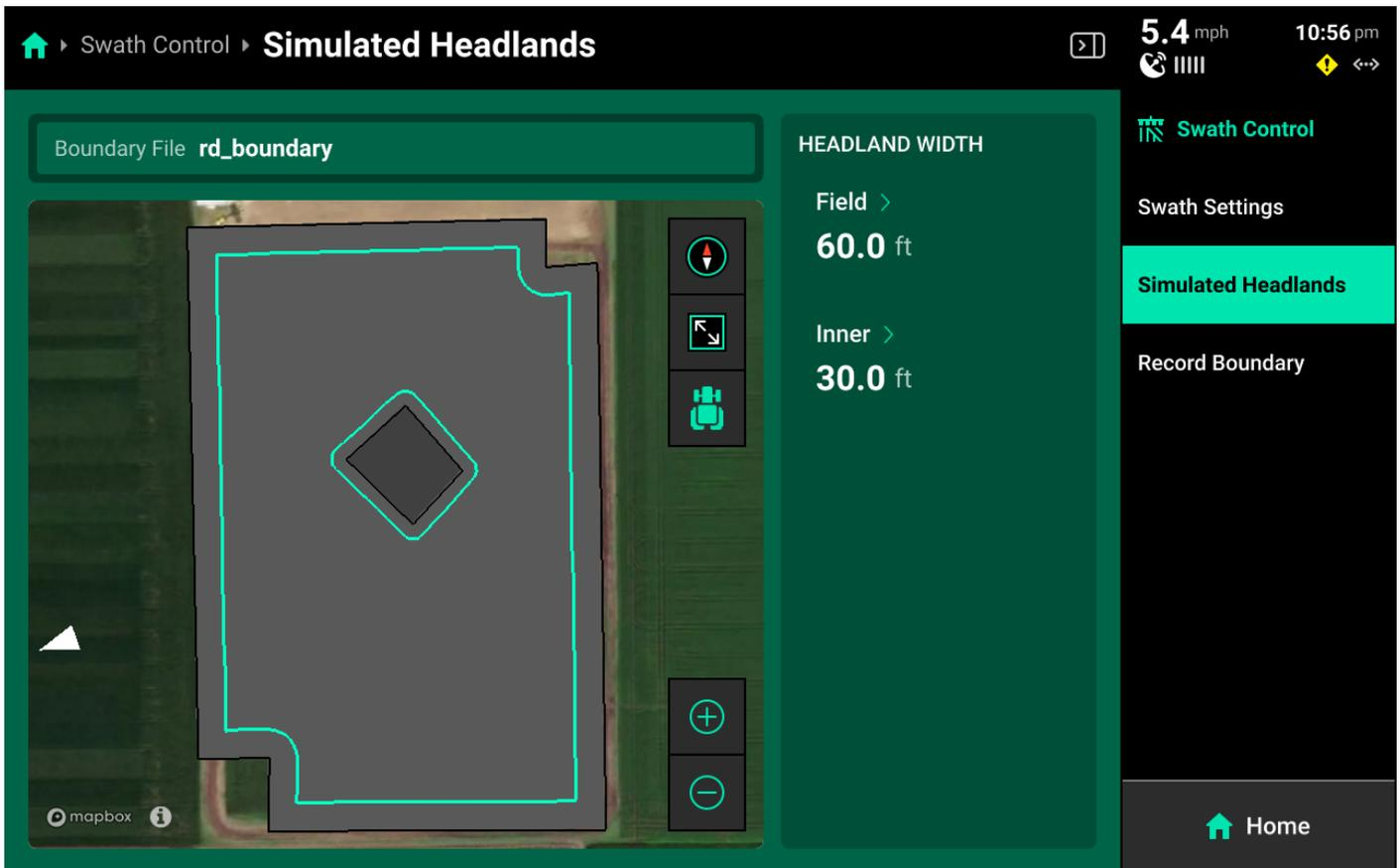
Select a width for Field (Exterior) or Inner to set the simulated headland width for either option.
