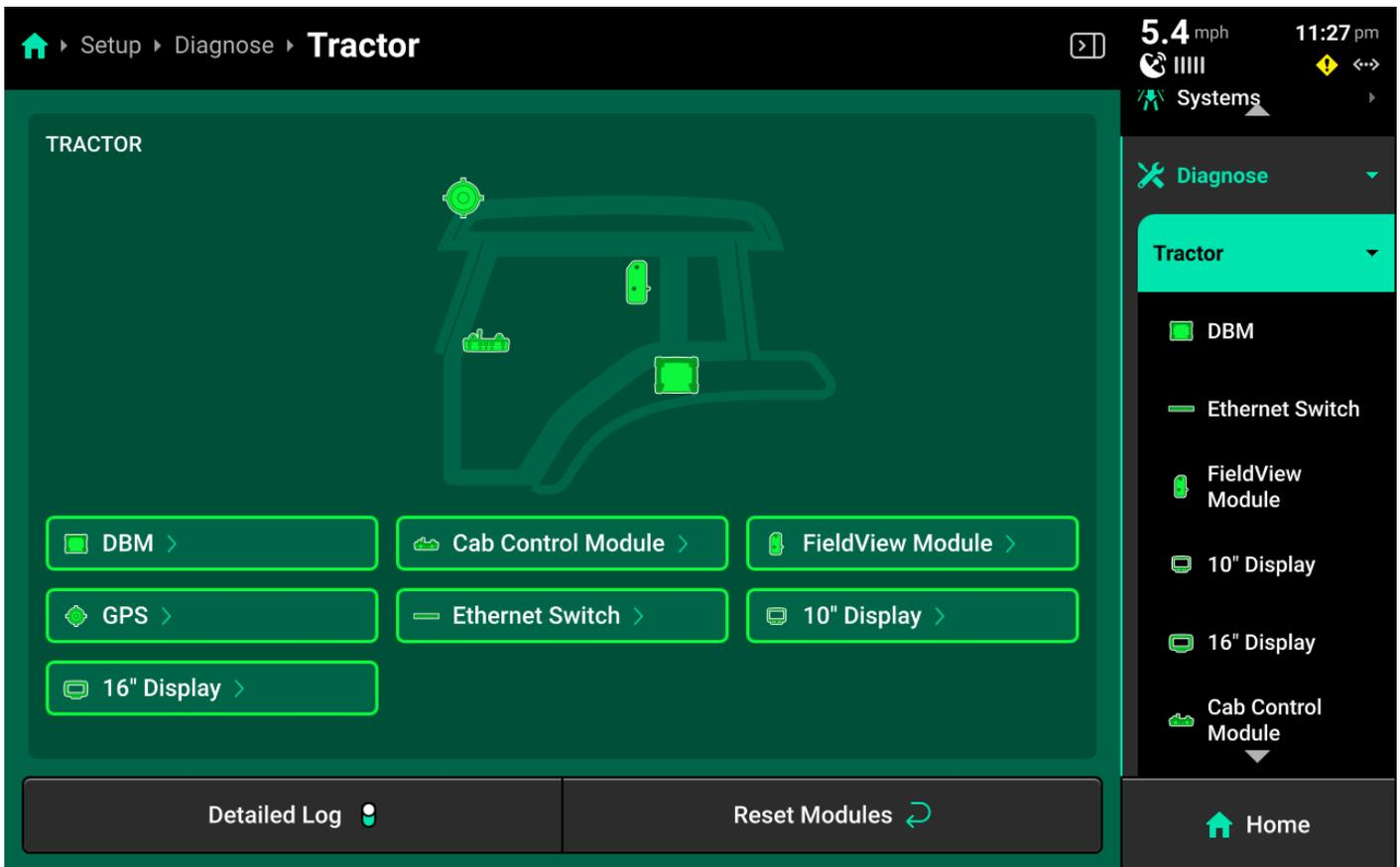
The **Cab** section of the diagnose menu will share the same name as the Cab profile that is selected in **Equipment**. A graphic of the Cab and all devices / modules that are installed on it will be displayed.
