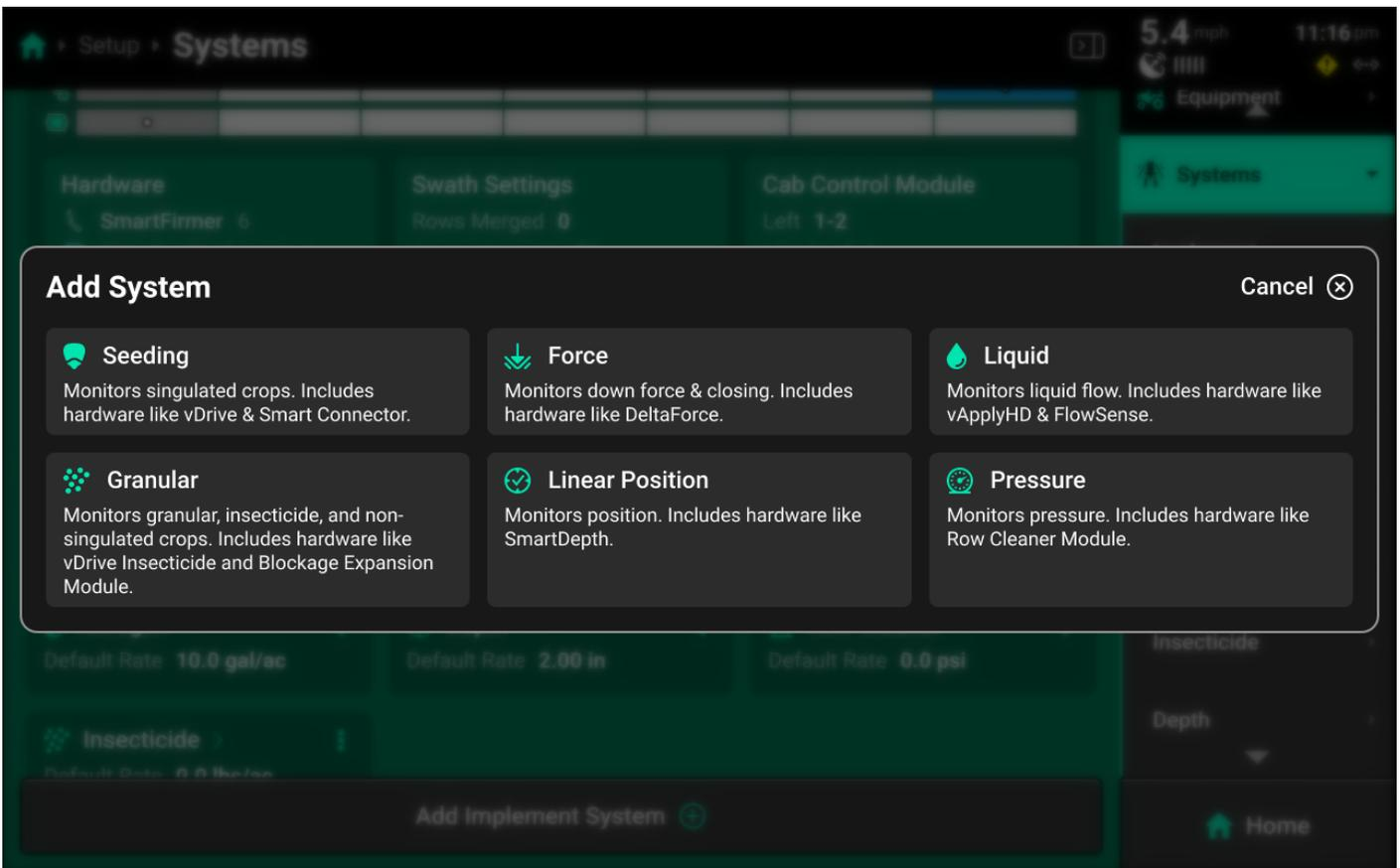
Selecting the type of system opens a second popup which allows the user to select a preset **Name** or enter a custom **Name**. It is advised to add all systems before proceeding to **Hardware Setup**.
