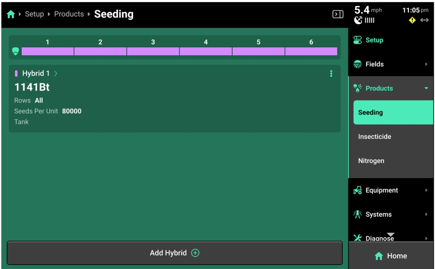
Press [**Seeding System Name**] under **Products** to add, delete or modify hybrids. A table of hybrid entries is displayed in the center. Press *Add Hybrid +* to immediately add a numbered hybrid entry to this table. Press the three dots next to any entry displayed in the table to delete it.
