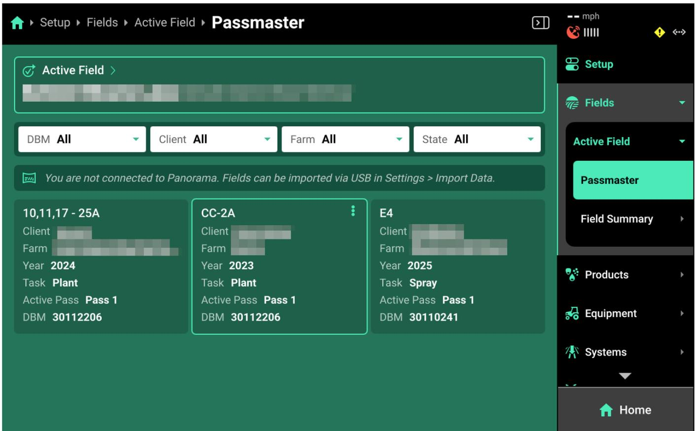
Press *Passmaster* under **Active Field** in the Navigation Menu to share field maps between multiple 20|20 monitors that are paired with the same Panorama operation. This is referred to as "**Subscribing**" to a pass. Data sharing is not limited to Coverage - all data will be shared. Data sharing is field-specific, the user must select what passes to share for each field on each DBM.
