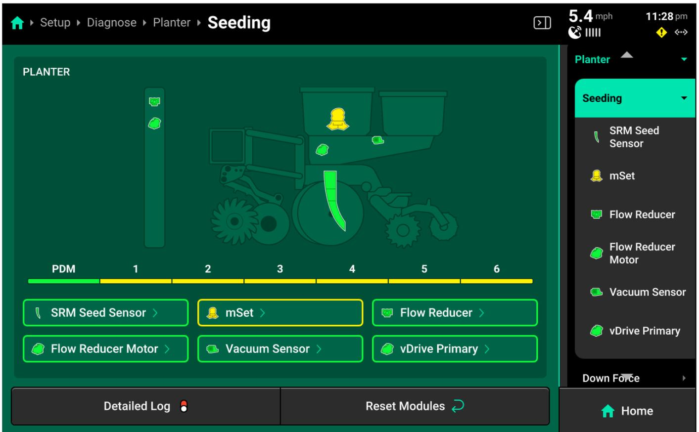
Press on the desired device to view a detailed diagnostic chart for that device.
