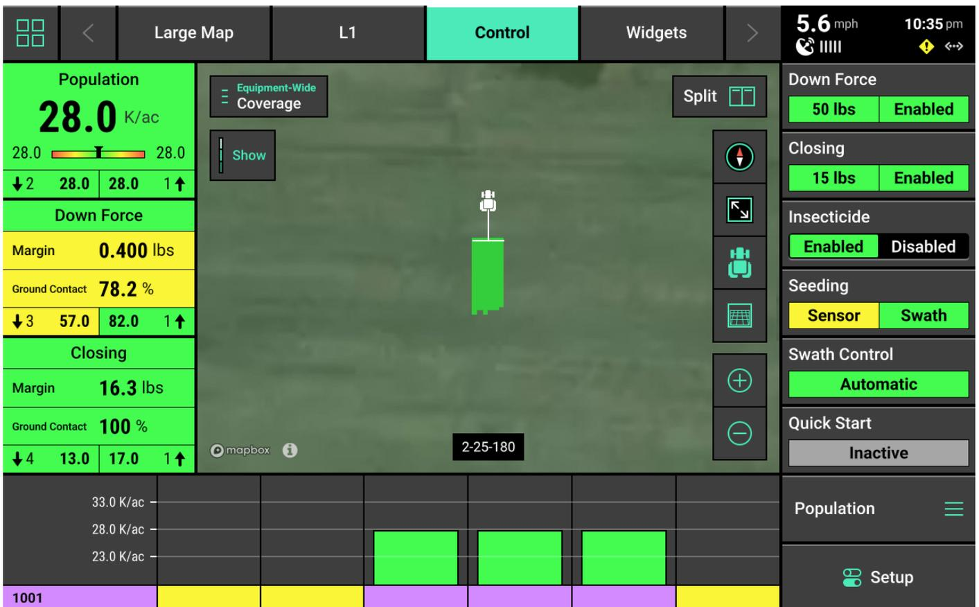
The name of the active metric shown on the DMC is displayed above the **Setup** button. To change
