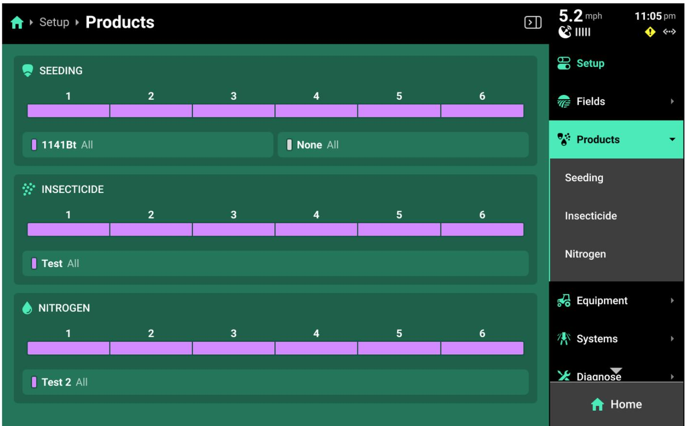
The **Products** menu is used to set up all hybrids and granular / liquid tank mixes. A list of seeding, liquid, and granular systems showing basic hybrid / tank mix information and indicating active rows for the hybrid / tank mix is shown on the **Products Landing Screen**.
