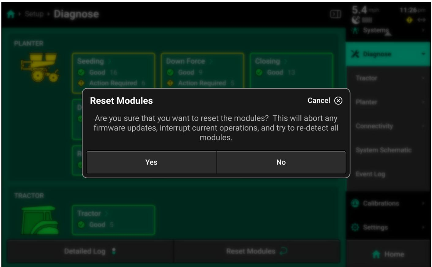
Press *Reset Modules* at the bottom and confirm on the popup to break and reestablish all CAN communication and daisy chain identification. This function is often used as a troubleshooting tool for communication issues.
