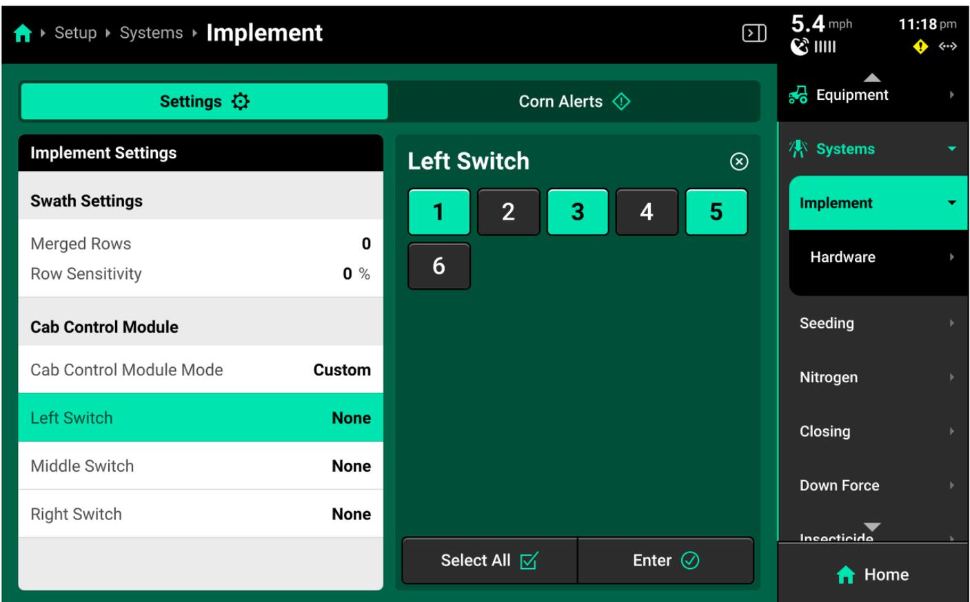
The left and right swath section switches are also used to Autoload any systems which have the auto load function enabled. Raise both switches up for one second to load systems. Systems with autoload enabled will dispense product. This allows product to immediately be dispensed when beginning to plant / apply. To continue autoloading, lift and hold both switches. Product will continue to dispense as long as the switches are held up.
