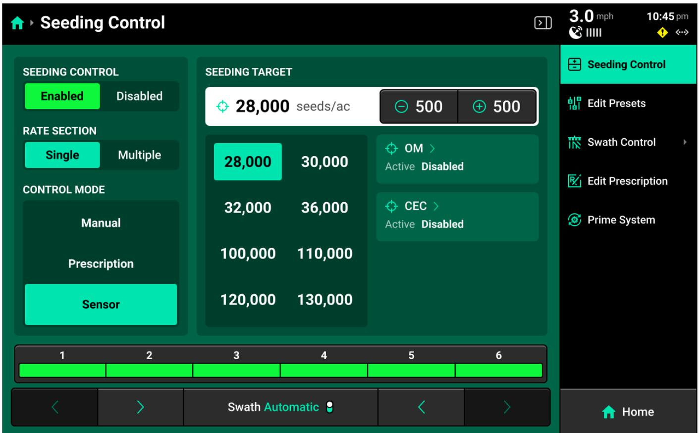
Some control systems may be configured to use a sensor to control rate. Sensors include SmartFirmers and Vision cameras. This guide details SmartFirmer sensor control setup. Refer to Vision documentation for information on setting up camera sensor control.
