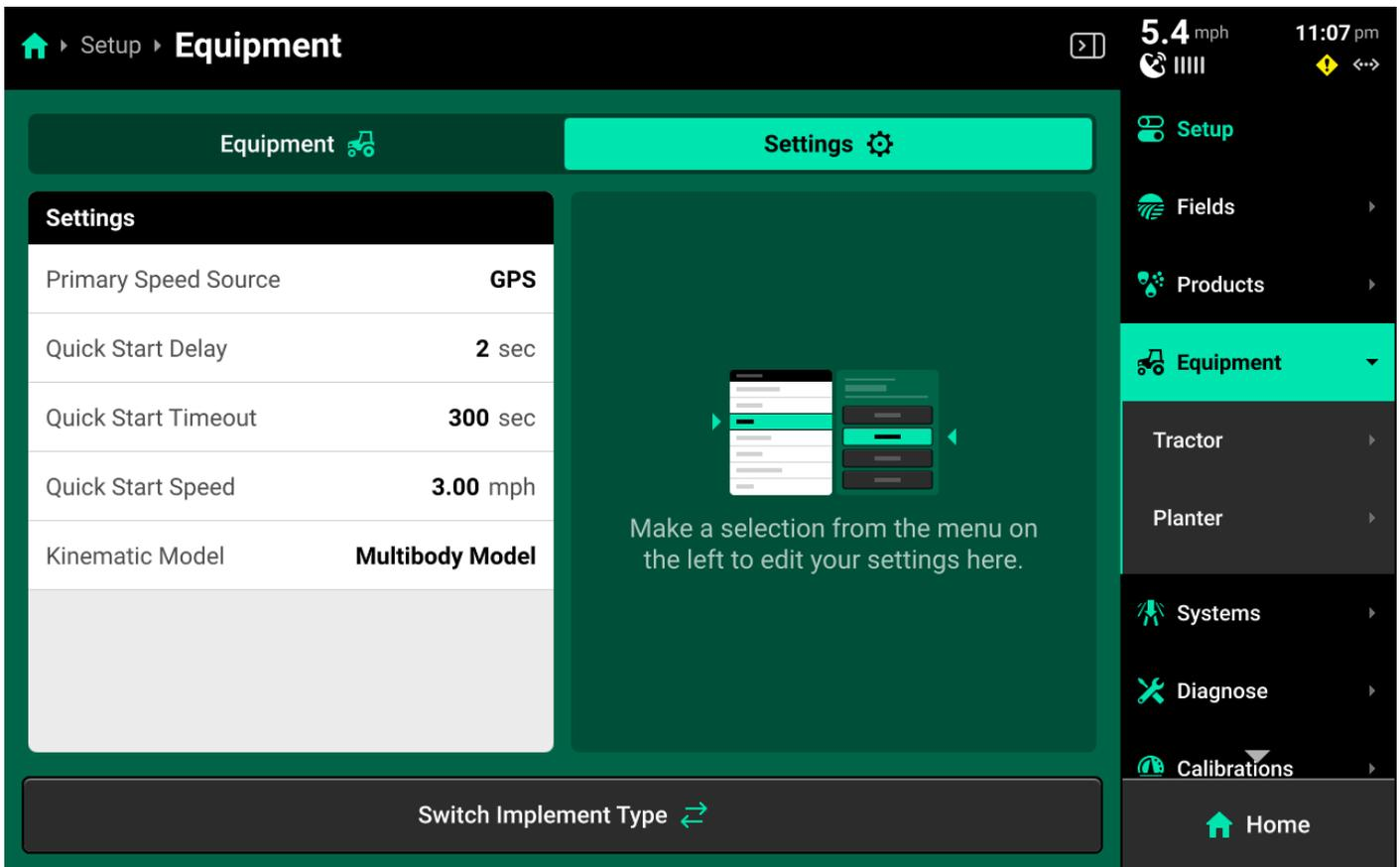
Use the tab at the top of the **Equipment Landing Screen** to select **Settings** for the Quick Start function. The Quick Start **Control Widget** will use the values from this screen when it is enabled. Quick Start allows the user to begin applying product at the simulated **Quick Start Speed** after the **Quick Start Delay** countdown. It will continue to run until either the **Quick Start Timeout** is reached, or until the 20|20 registers speed from the **Primary Speed Source**.
