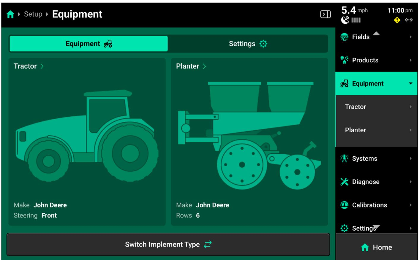
The **Equipment** menu is used to configure, save, and load different Cab or Implement profiles. Use this menu to enter all Cab / Implement specifications and measurements, to configure GPS and Radar location and settings, and to set up Ethernet / CAN.
