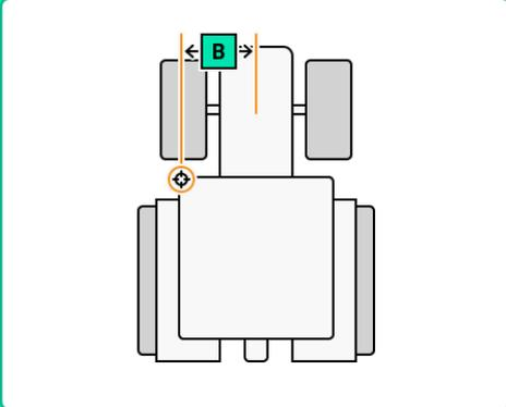
Enter the distance from the center of the tractor to the center of the GPS
