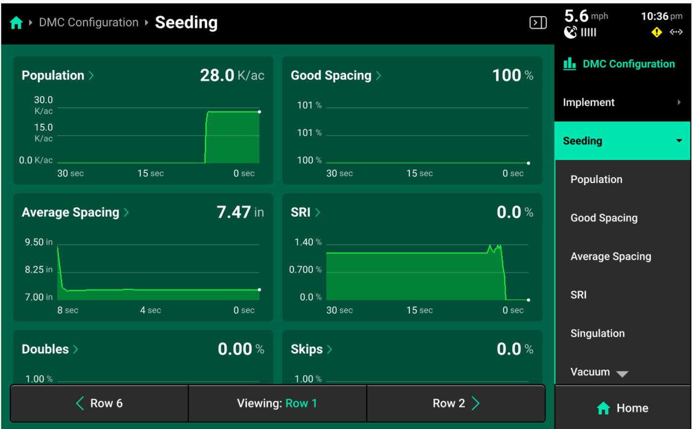
Press *DMC Configuration* in the upper right to toggle DMC Auto Scroll on or off, or to adjust the scroll frequency that the DMC will use when cycling between metrics. If Auto Scroll is set to single, change the displayed metric by selecting it in the table in the right window.
