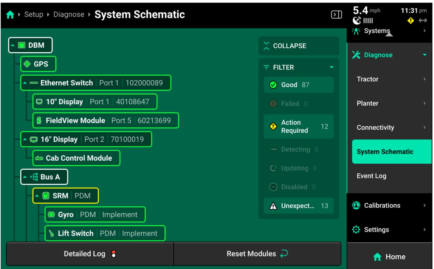
For any device that has a dropdown arrow next to its icon, press that arrow to expand the schematic to show all connected devices. Alternatively, press *Expand* in the upper right corner to immediately expand the entire schematic.
