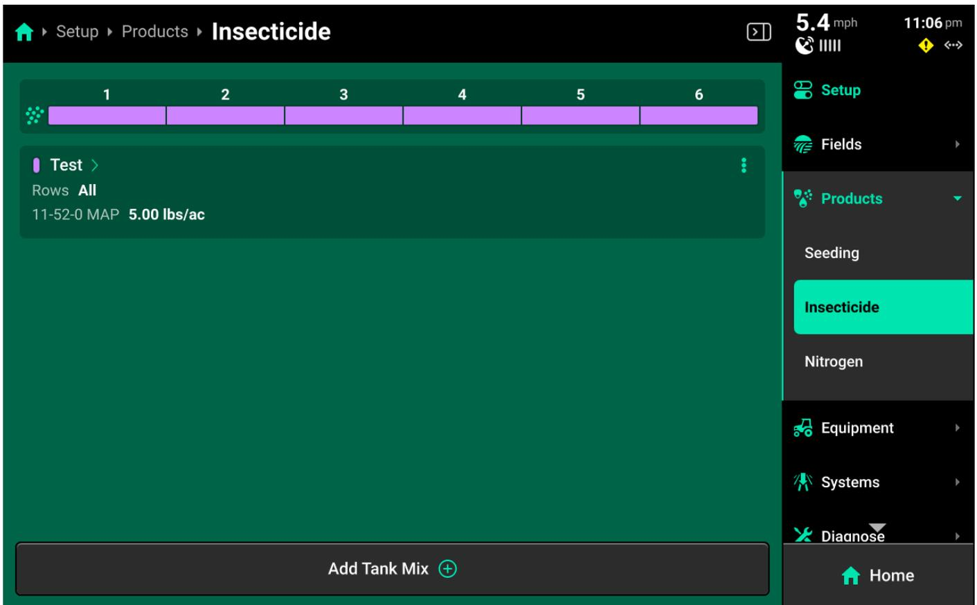
Press any of the liquid or granular systems under **Products** to add, delete, or modify tank mixes. A table of all tank mixes for the selected system is displayed in the center. Press *Add Tank Mix +* and enter the desired name for the tank mix. A new tank mix will then be displayed in the table.
