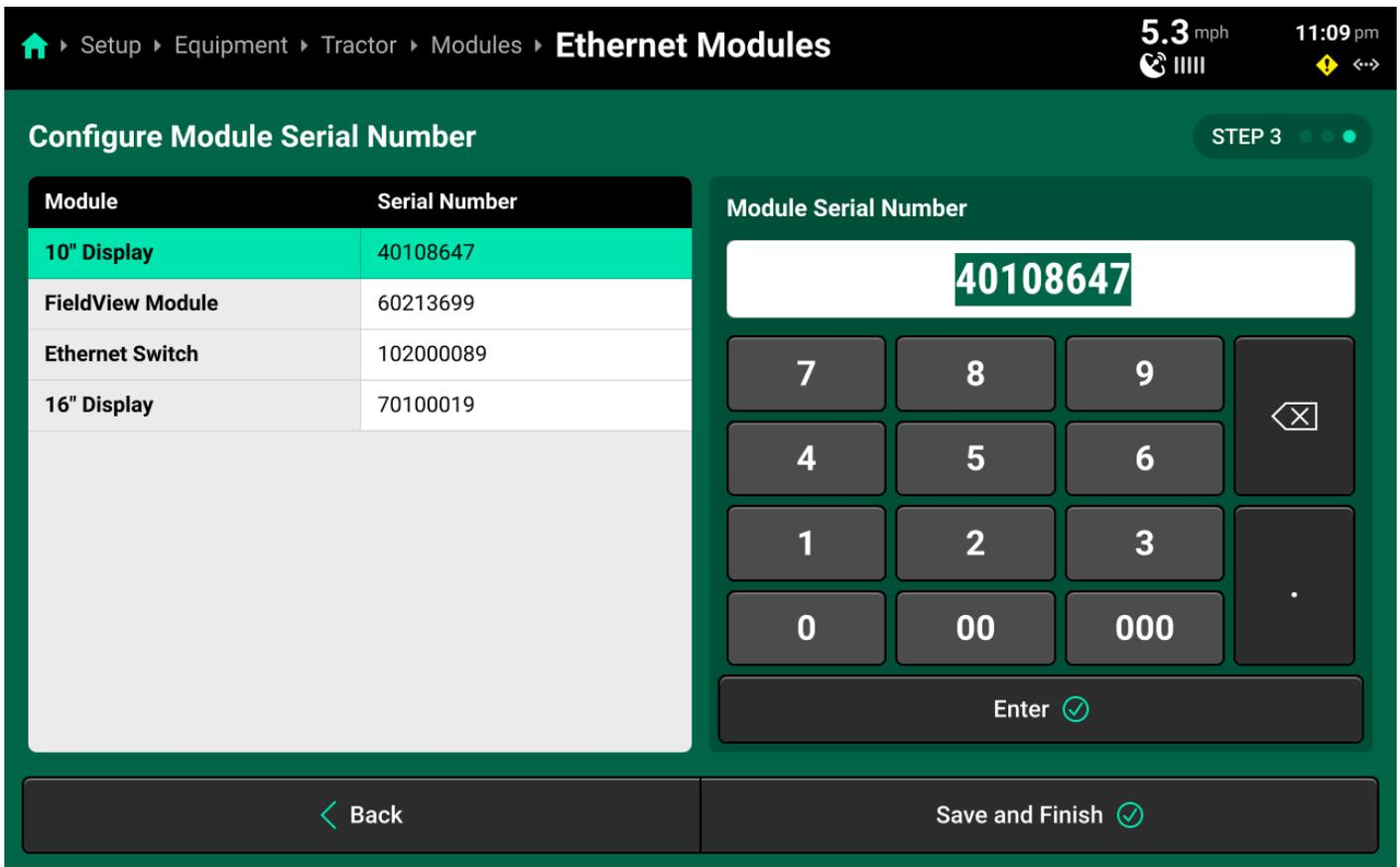
Confirm or enter correct serial number for each device on **Step 3**. Press *Save and Finish* to exit setup and return to Modules. Ensure that Ethernet devices are listed correctly below DBM in the left window.
