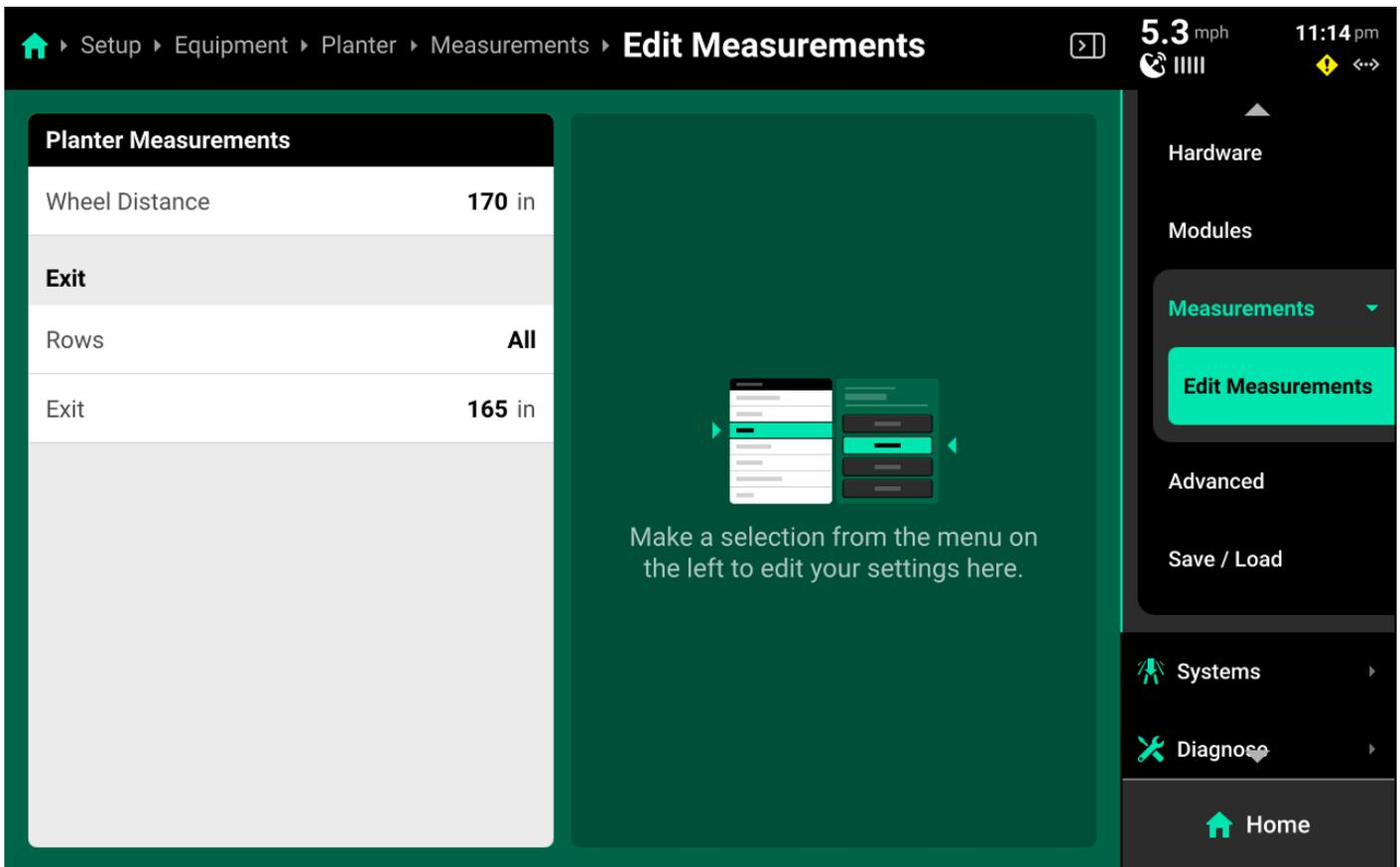
Select the desired dimension in the left window and use the right window to modify the dimension. Some dimensions will expand in the left window when pressed to display a graphic indicating what to measure. Continue scrolling after entering a value to view all available dimensions.
