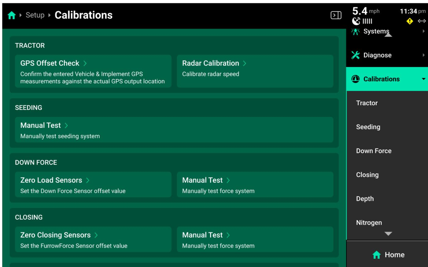
A master list of available calibrations will be displayed on the **Calibrations Landing Screen**. Filter this list by pressing on the options displayed below **Calibrations** in the Navigation Menu.
