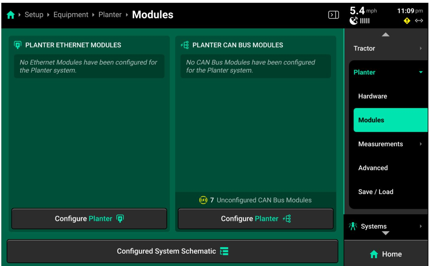
Use the **Modules** screen to set up Ethernet layout and serial numbers, and CAN module sequence and location.
