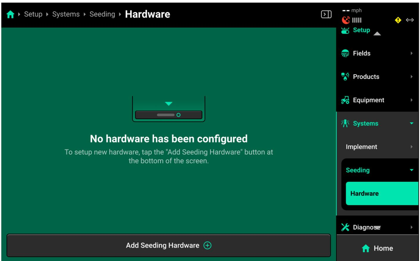
Press *Hardware* below each system in the Navigation Menu to set up that system's hardware. Press *Add (System Name) Hardware* at the bottom to open a popup which allows the user to select the desired hardware device.
