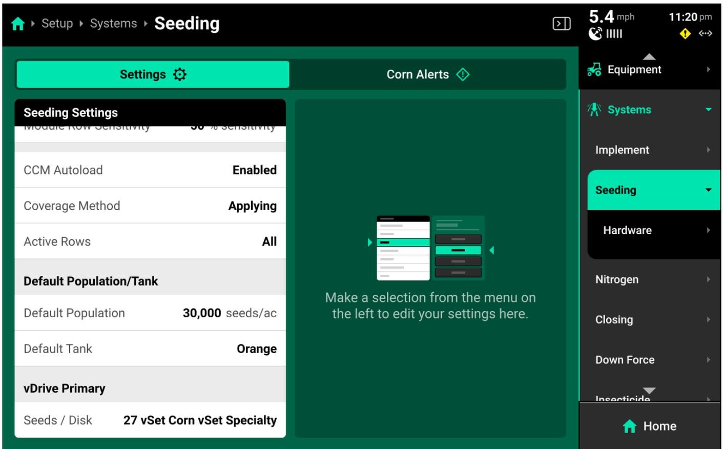
Some Operation Settings (e.g. vDrive seeds / disk) are also available under the **System Settings** tab on the **Field Setup** screen.
