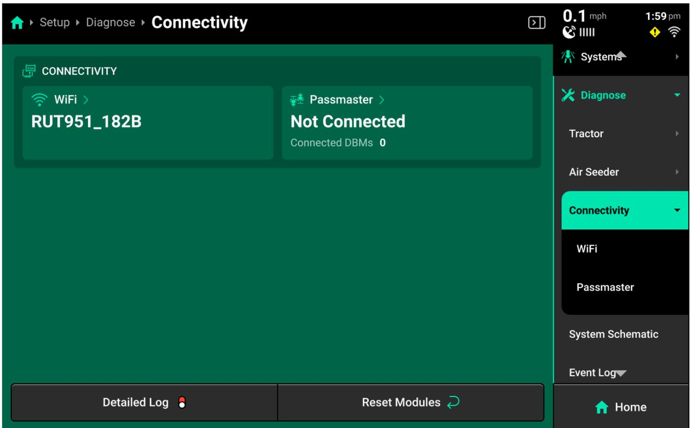
The **Connectivity** section of the Diagnose menu displays Wi-Fi and Passmaster connection status. Press on either option in the center or Navigation Menu to view each connection details.
