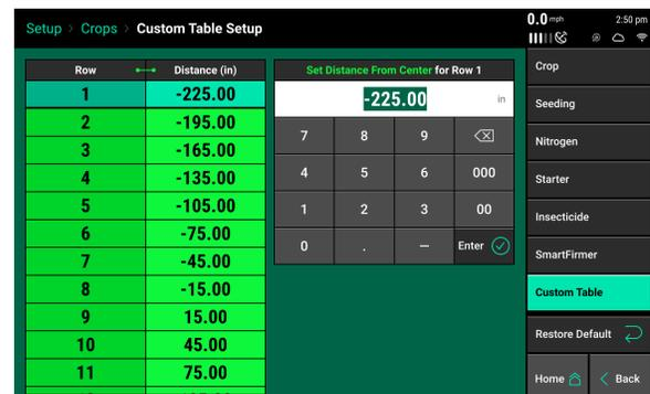
For each row number, set the “Distance from Center” number for each row and select enter after entering the distance before moving to the next row. Distance set in the Custom Table Setup will be reflected in the Frame Layout found in the Equipment menu.
