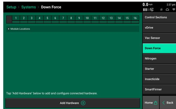
Press 'Add Hardware' at the bottom of the screen to begin the setup process. Assign what rows have a down force sensor installed, and press 'Done'.
