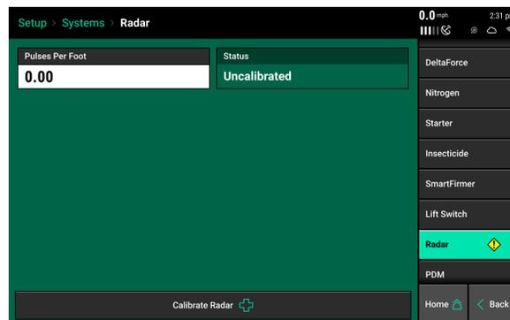
The calibration process will require a good GPS signal as well as having the operator drive straight for at least 300 feet at a constant speed of 4 mph or greater.
