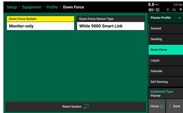
Navigate to Setup — Systems — Down Force to configure the down force sensors.
