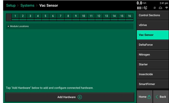
Press 'Add Hardware' at the bottom of the screen to begin the setup process. Assign what rows have a vac sensor installed, and press 'Done'.
