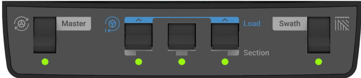
The switch on the left hand side is the Master Plant switch. For all control products to function the Master Plant switch must be in the up position. If it is in the down position, all control products will immediately be disabled.
