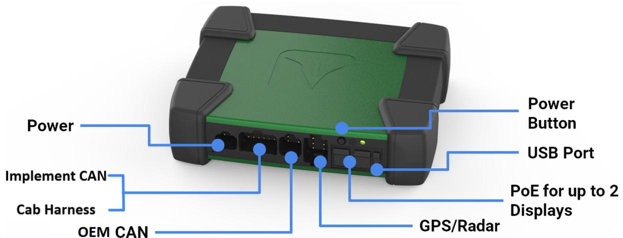
The Power over Ethernet [PoE] ports requires a Shielded Twisted Pair [STP] Ethernet Cable to connect to a display. If only one display is being used, use either port. Both ports will be used if connecting to two displays or one display and a FieldView Module [FVM]. The order by which two displays or a single display and FVM are plugged in does not matter.
