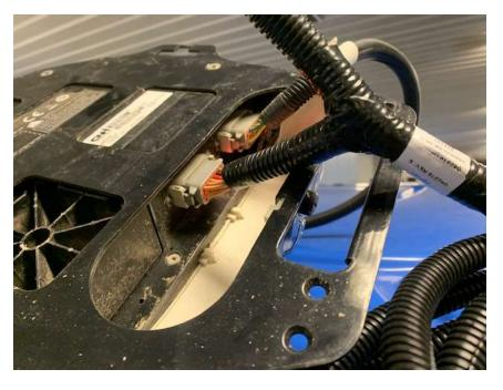
**Step 3:**Reinstall the receiver on the cab and route the adapter harness into the cab to plug into the 4–pin GPS connection on the speed/cab harness of the 20|20
