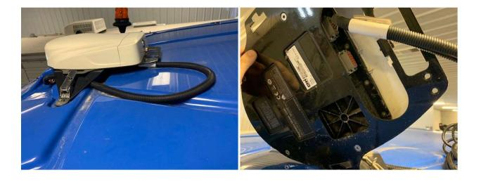
**Step 2:** Using the 727131 sdapter harness, plug the 12–pin Deutsch plug into the opne port #2 in the back of the receiver
