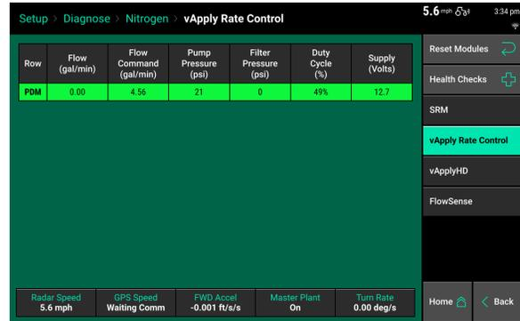
The screenshot shows the 'vApply Rate Control' diagnostic screen. At the top, the breadcrumb path is 'Setup > Diagnose > Nitrogen > vApply Rate Control'. The main area contains a table with the following data:
