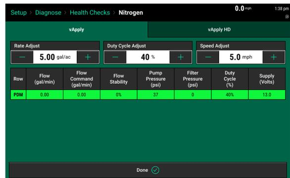
The Manual test has multiple tabs at the top that allow you to view various information. The tab for vApplyHD shows the vApplyHD module information. If FlowSense is installed, the tab for FlowSense will show FlowSense information.
